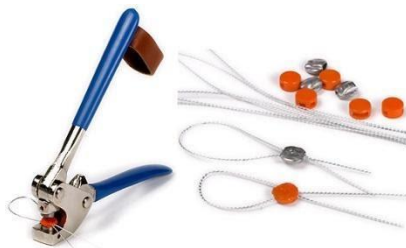
Figure 8. Sealing stamps and pliers used for pressing the seals.
